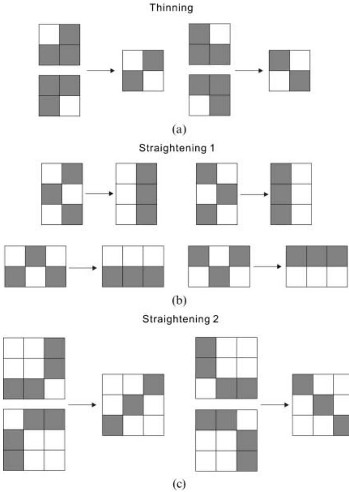
Figure 5. Posteriorization procedures of thinning and straightening for improving the final shape of a path: (a) thinning; (b) straightening 1; (c) straightening 2.
