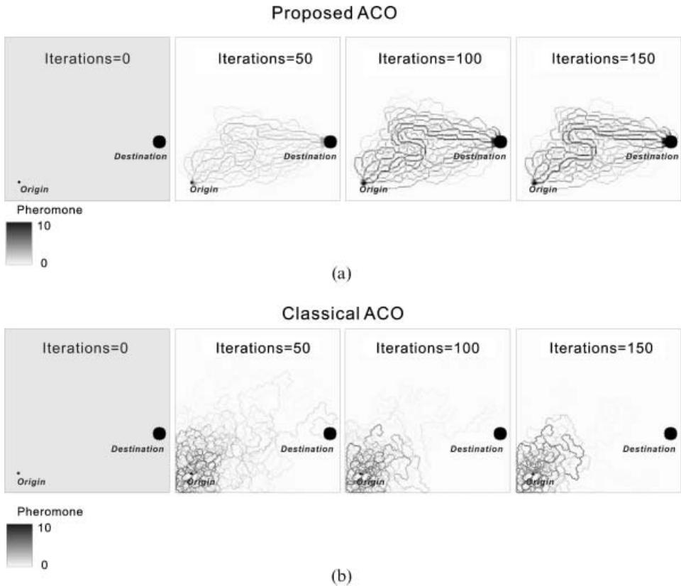
Figure 11. Optimal path formation based on pheromone updating: (a) proposed ACO; (b) classical ACO.
