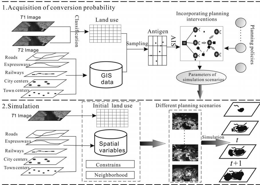
Figure 1. AIS-based CA model for urban planning.
